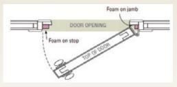
is to look for sunlight through the cracks. When you approach a door, look at the seals when it is a bright and sunny day. Notice if you can see light seeping through or illuminating the seam. If you do, the seal is not airtight.
